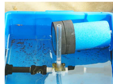
Remove the float to stop irrigating
