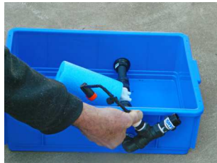
Connect the adjustable control dripper
