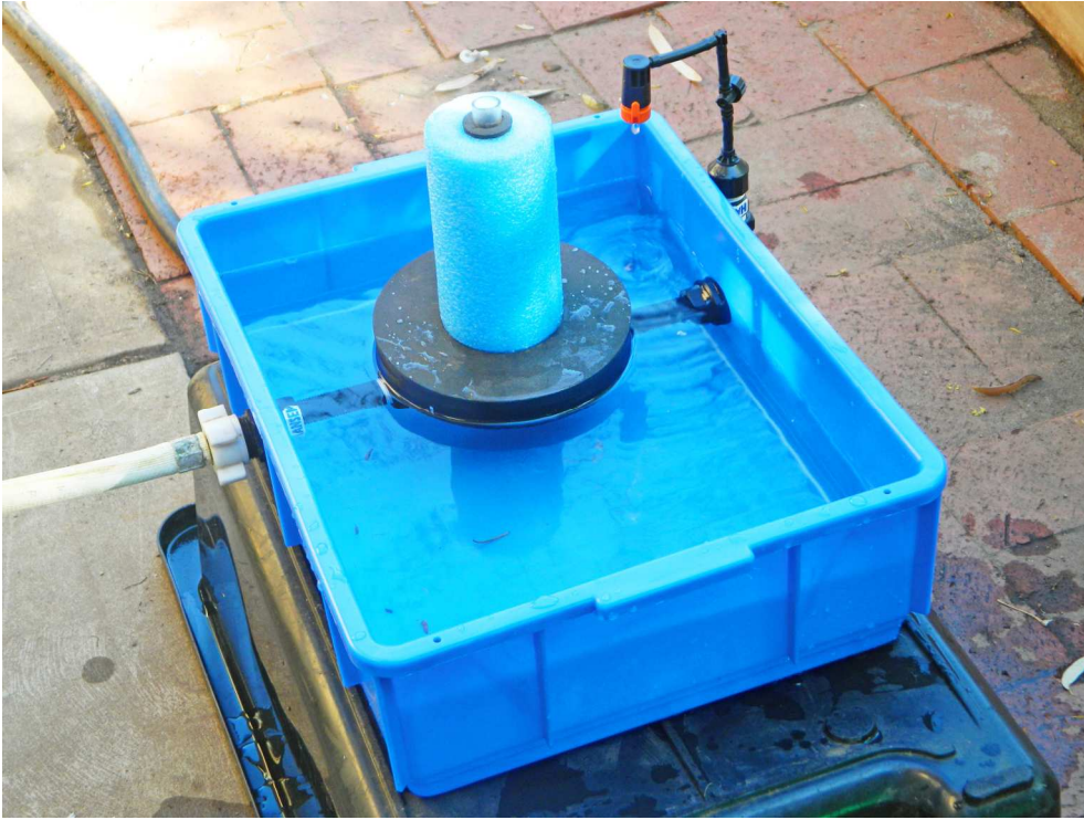
Unpowered Evaporative Valve
