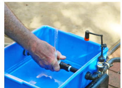
Float shaft must be vertical
