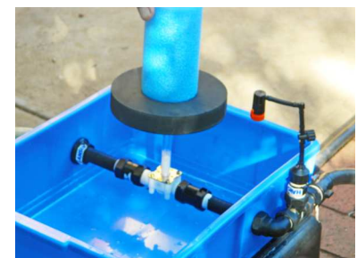
Slide the float over the float shaft
