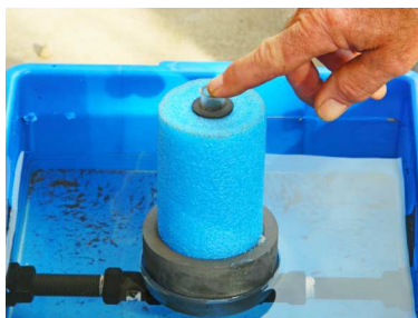
Push the float down to start irrigating
