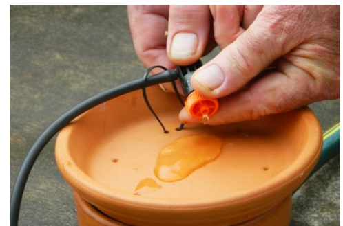
The control dripper is adjustable.
