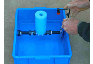
Tighten the two back-nuts
