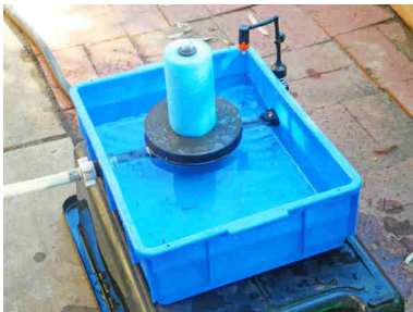
The irrigation starts when the float reaches the low level
