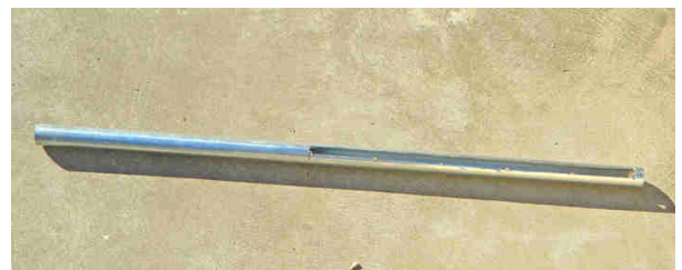
An angle grinder can be used to make a long slot in a length of steel pipe
