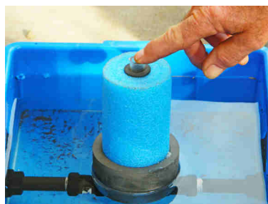
Push the float down to start irrigating
