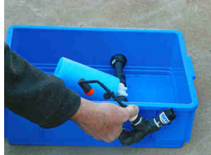
Connect the adjustable control dripper
