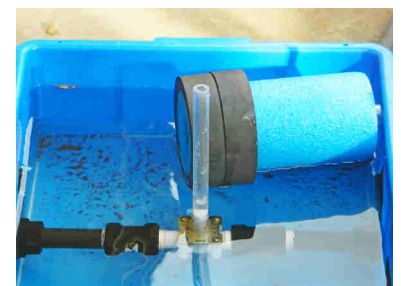
Remove the float to stop irrigating
