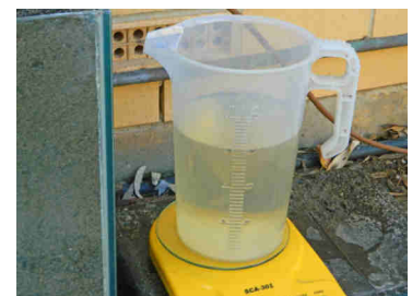
Reweight the container to determine the volume of water that has evaporated
