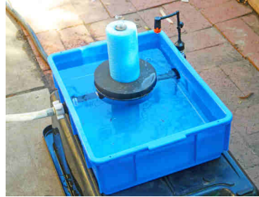
The irrigation stops when the float reaches the high level
