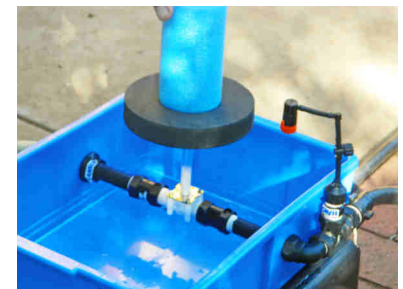
Slide the float over the float shaft
