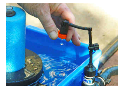
Adjust the control dripper
