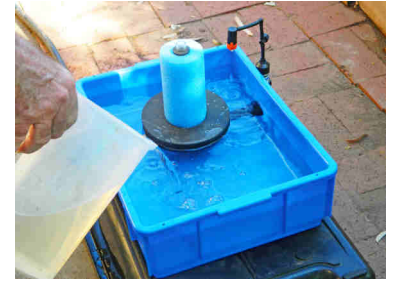
Fill the evaporator with water until the irrigation stops
