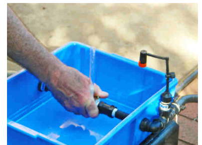
Float shaft must be vertical
