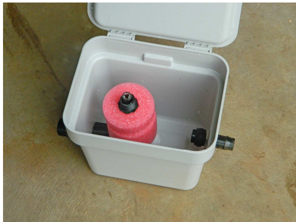
Float inside Unpowered Wicking Bed Controller
