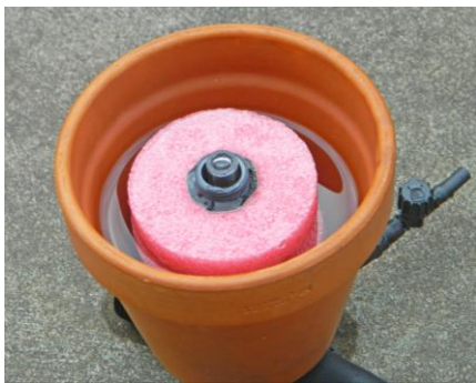
Unpowered Terracotta Valve showing the float and the water level
