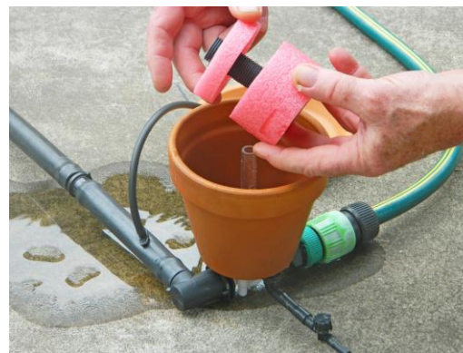
To adjust the interval between irrigation events, adjust the gap between the upper and lower floats
