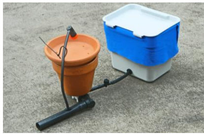
Booster connected to the drain valve on the terracotta pot
