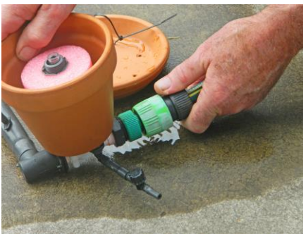
Connect the water supply to the valve inlet
