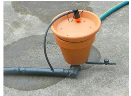
Place the terracotta saucer on the terracotta pot so that the control dripper drips water into the pot
