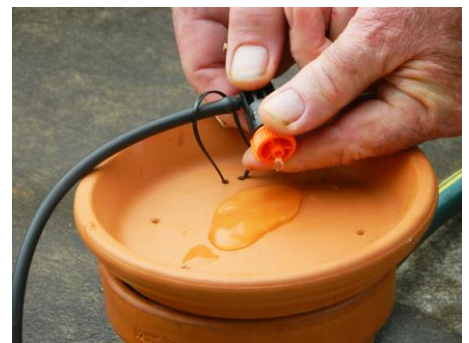
The control dripper is adjustable.
