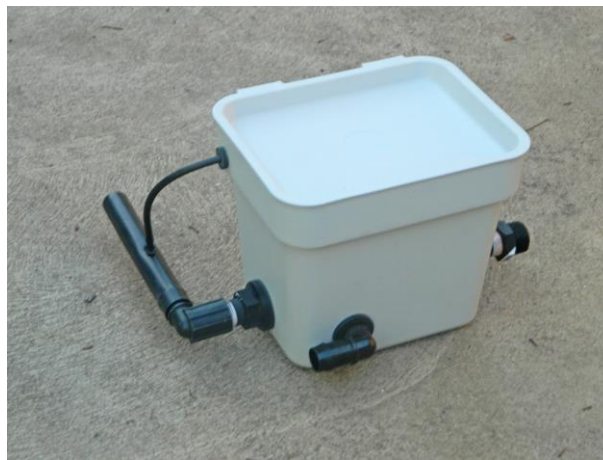
Unpowered Valve Box
