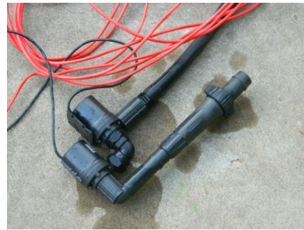
Double pump (two 19 watt pumps connected in series) with an inlet filter, fittings to connect to 19 mm poly pipe, and 9 metres of waterproof electrical cable
