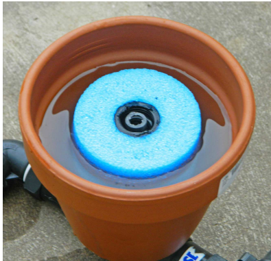
Unpowered Terracotta Valve showing the float and the water level
