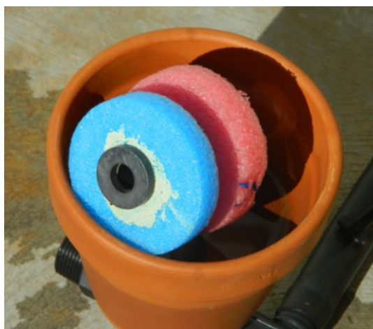
Float showing the ring magnet at the bottom of the float
