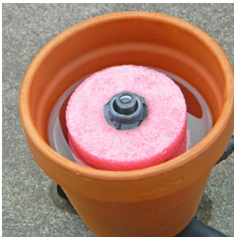
Unpowered Irrigation Controller showing the float and the water level
