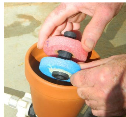
To adjust the interval between irrigation events, adjust the gap between the upper and lower float
