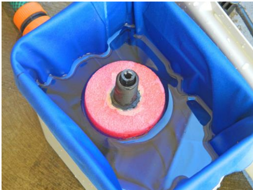
Unpowered Wicking Irrigation Controller showing the float and the water level
