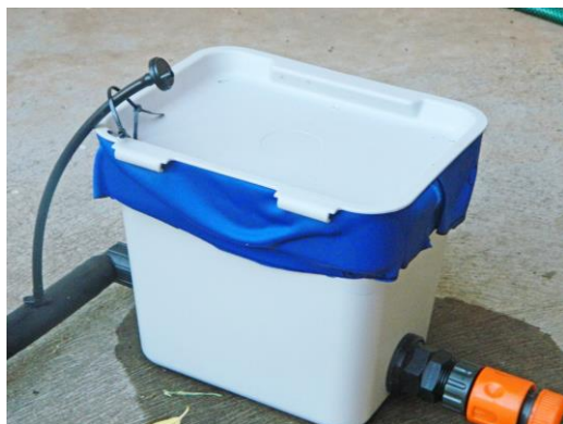
To increase the interval between irrigation events, reduce the surface area of exposed fabric
