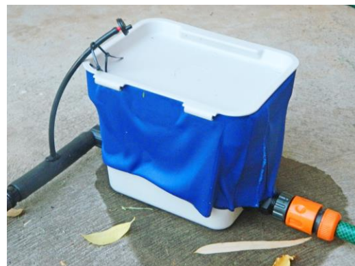
To reduce the interval between irrigation events, increase the surface area of exposed fabric
