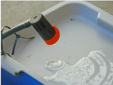
Position the control dripper so that it drips water into the container
