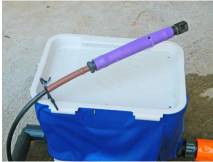
The control dripper may be one or two irrigation drippers
