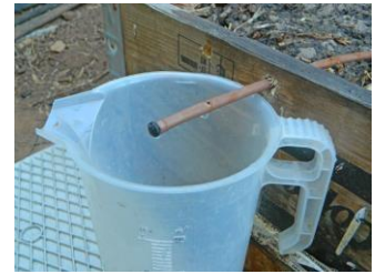
Position a measuring container under one of the irrigation drippers
