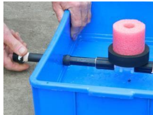
Slide the cylindrical float over the float shaft
