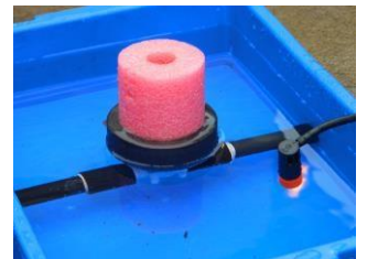
Position the control dripper so that water drips into the evaporator
