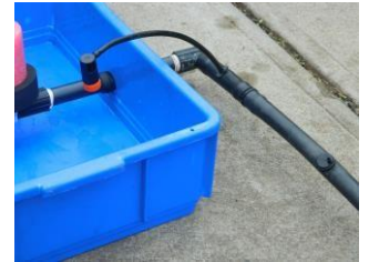
Connect the irrigation application to the outlet side of the evaporator
