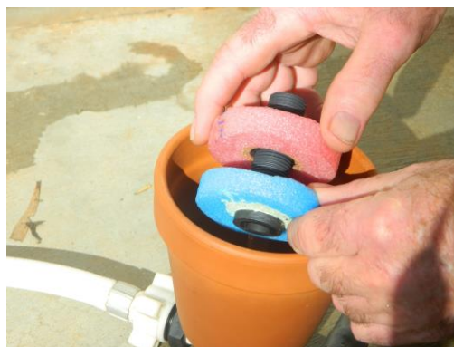
To adjust the interval between irrigation events, adjust the gap between the upper and lower float
