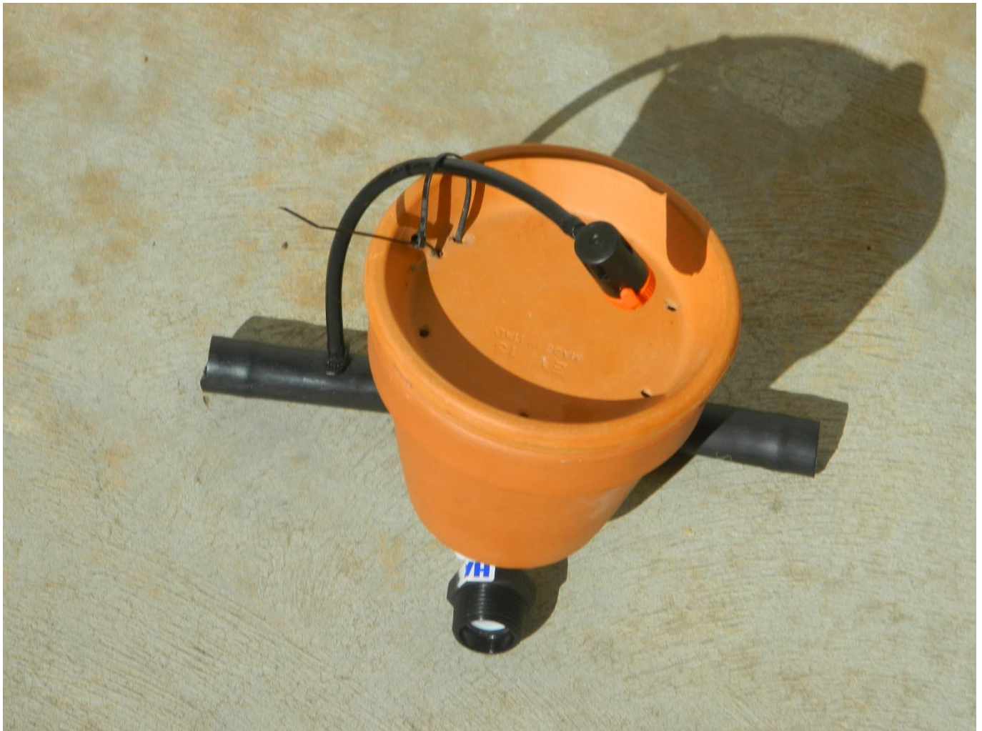
Unpowered Irrigation Controller
