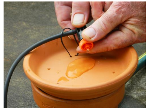
The control dripper is adjustable.
