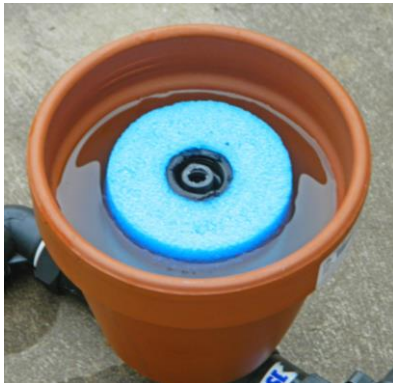
Unpowered Irrigation Controller showing the float and the water level
