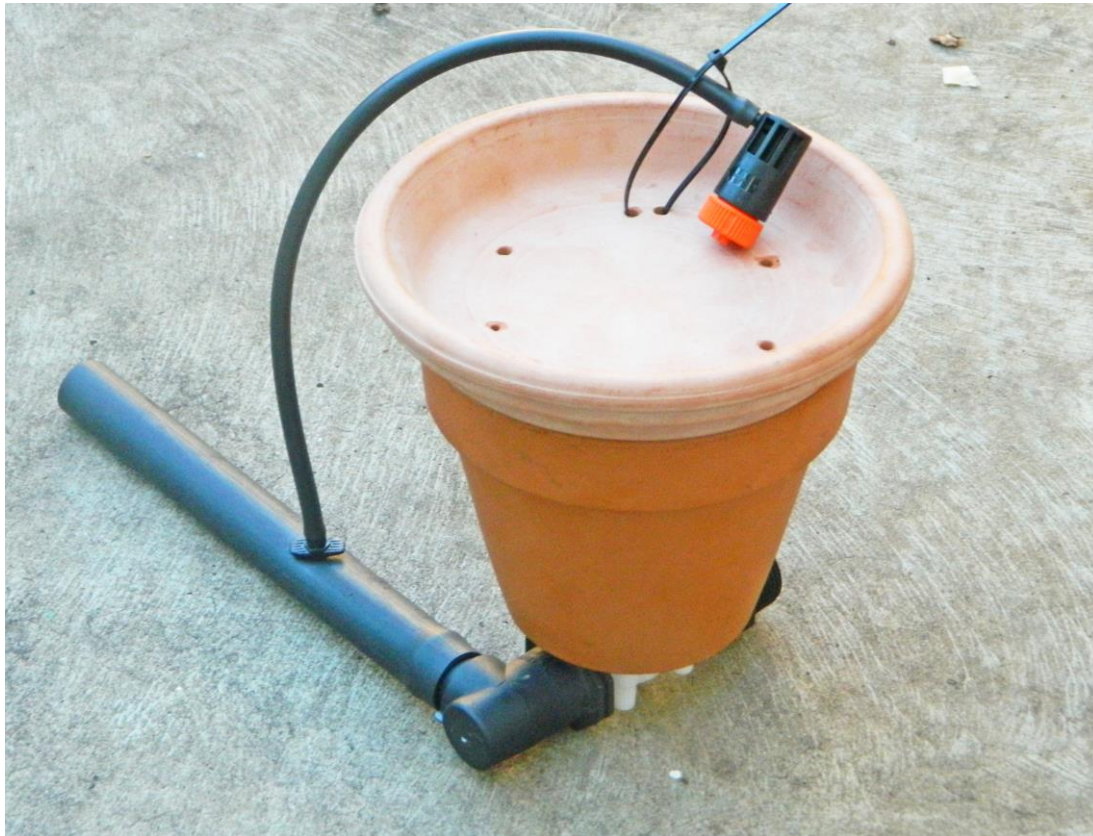
Unpowered Irrigation Controller
