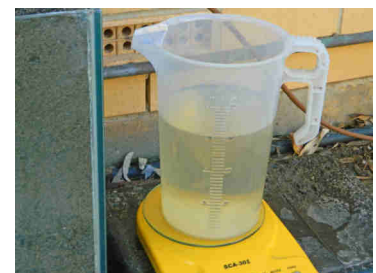
Reweigh the container to determine the volume of water that has evaporated
