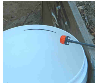
The adjustable dripper drips water into the evaporator during the irrigation event
