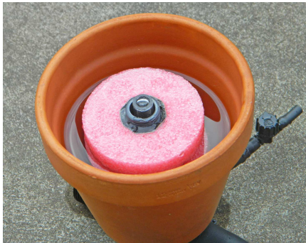
Unpowered Terracotta Valve showing the float and the water level
