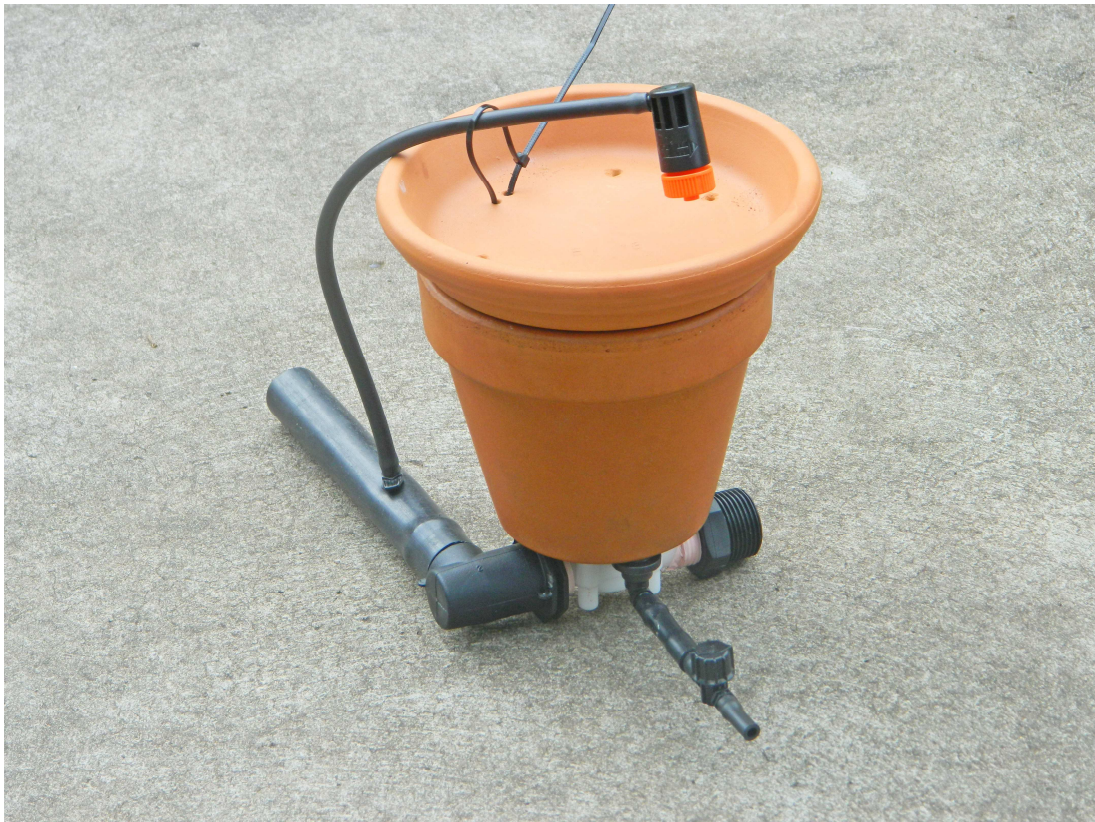
Unpowered Terracotta Valve
