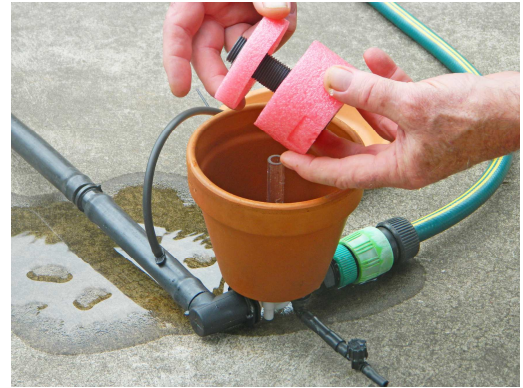
To adjust the interval between irrigation events, adjust the gap between the upper and lower floats
