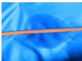
Polyester fabric starting to wet under dripper
