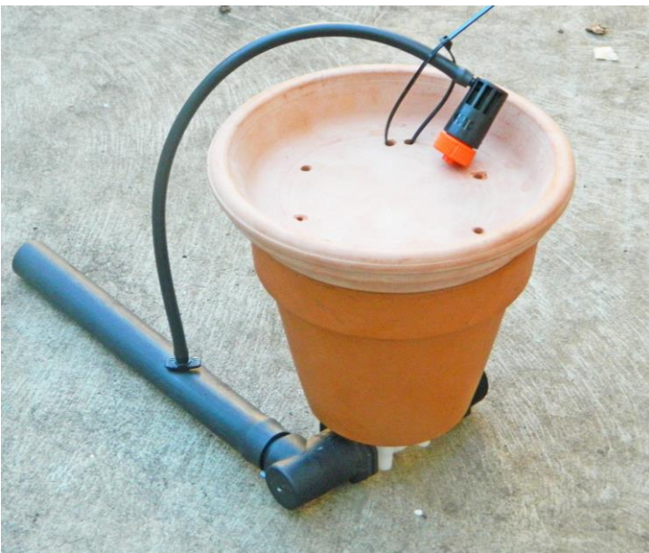
Unpowered Terracotta Irrigation Controller
