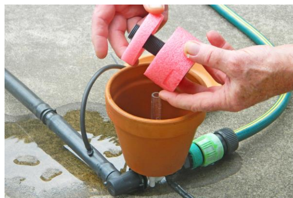
To adjust the interval between irrigation events, adjust the gap between the upper and lower float
