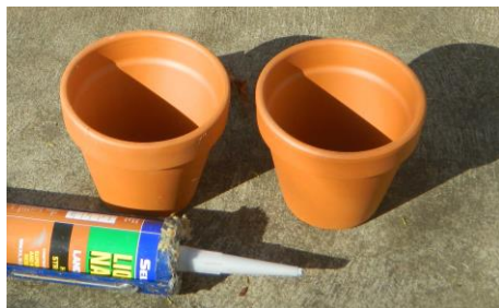
Step 1. Select two identical unglazed terracotta pots and seal one of the drain holes (for example, use silicone adhesive or masonry adhesive)
