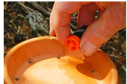
The control dripper is adjustable.
