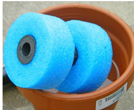
Float showing the ring magnet at the bottom of the float
