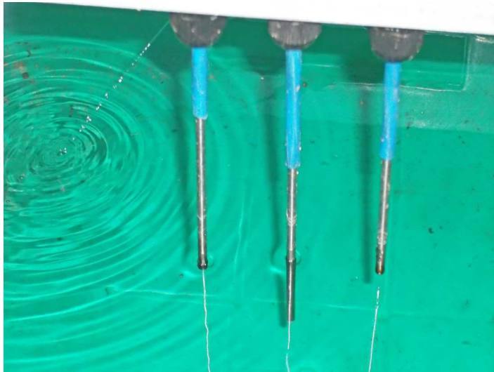
Fig. 3 Level sensor with the low probe on the left (in the water), the reference probe in the middle, and the high probe on the right (out of the water)
