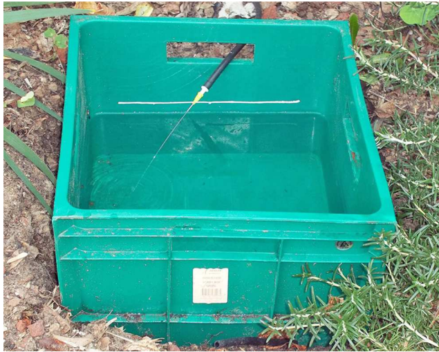
Fig. 2 Yellow control nozzle delivering water to the evaporator
