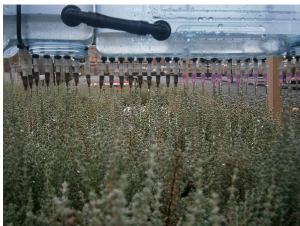
Fig. 8b Emitter nozzles for boom irrigation
