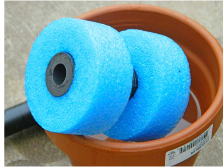
Float showing the ring magnet at the bottom of the float
