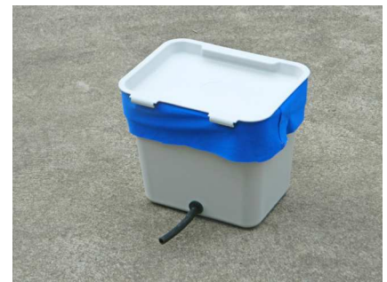
Adjust the interval between irrigation events by adjusting the exposed surface area of polyester cloth
