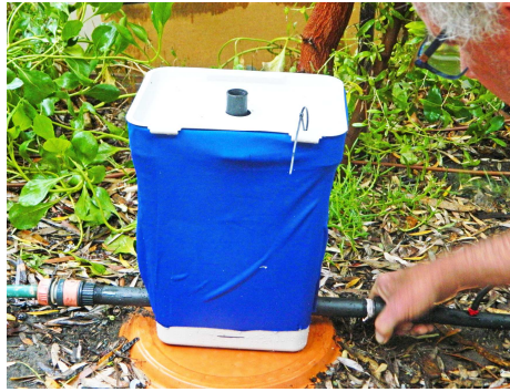
Connect the irrigation application to the valve outlet
