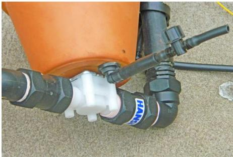
Drain valve and white valve with 15mm inlet and outlet
