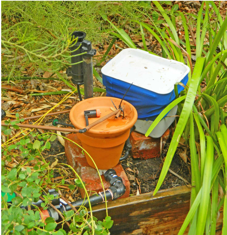
Terracotta Irrigation Controller for Latching Solenoids with Control Volume Boost Container
