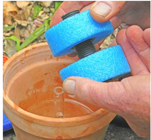
To adjust the interval between irrigation events, adjust the gap between the upper and lower floats
