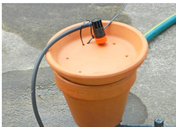
Place the terracotta saucer on the terracotta pot so that the control dripper drips water into the pot
