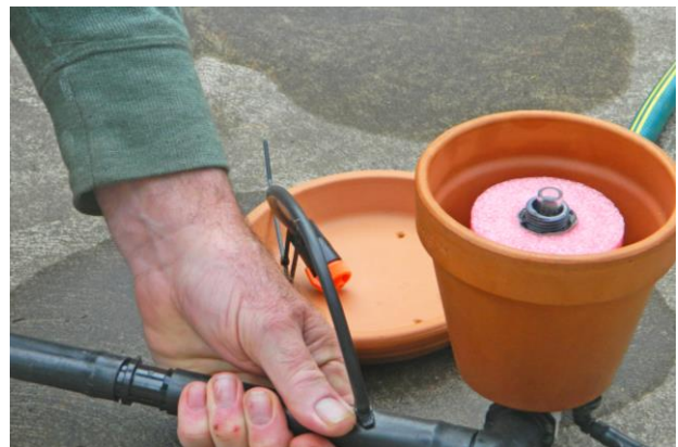
Connect the irrigation application to the valve outlet
