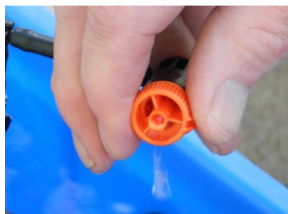
Adjusting the control dripper
