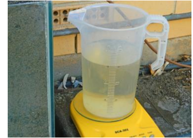
Reweigh the container to determine the volume of water that has evaporated
