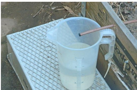
Check the volume of water in the measuring container.
