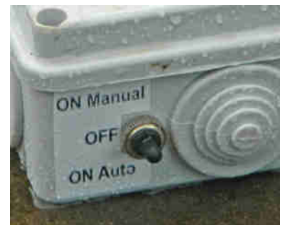
Switch with 3 positions: ON Manual, OFF, ON Auto
