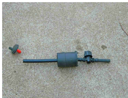
Step 2. Insert the 4mm polypipe through the hole in the end plug.
