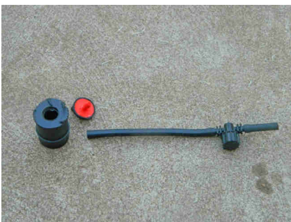
Step 1. Connect 4mm polypipe to the 4mm micro valve. Drill a 13mm hole in the 25mm end plug.
