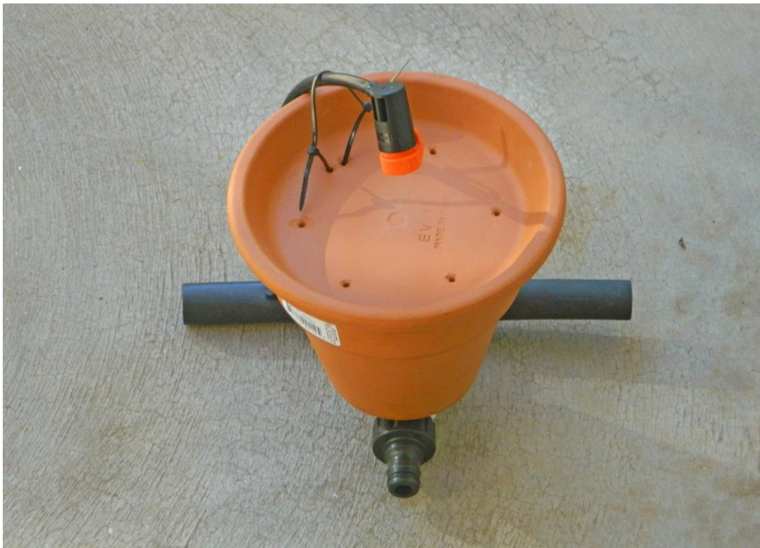
DIY Unpowered Terracotta Irrigation Controller
