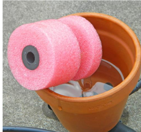
Float showing the ring magnet at the bottom of the float
