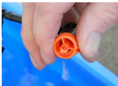
Adjusting the control dripper
