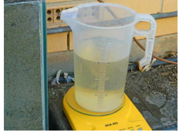
Reweight the container to determine the volume of water that has evaporated
