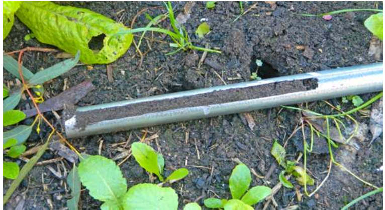
Remove the steel pipe from the soil and use the slot to inspect the moisture level in the soil and the position of the wetting front.
