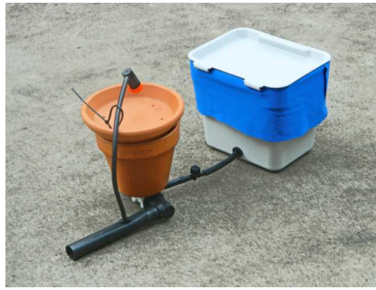
Control Volume Boost Container connected to the drain valve on the terracotta pot
