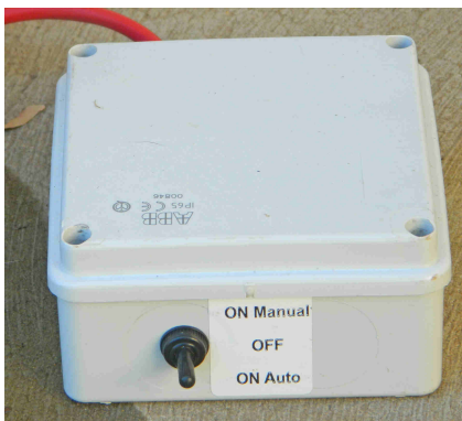
Waterproof pump controller with solar charge controller inside
