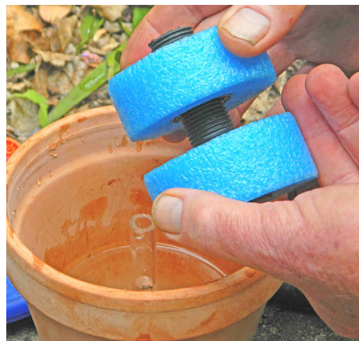
To adjust the interval between irrigation events, adjust the gap between the upper and lower floats
