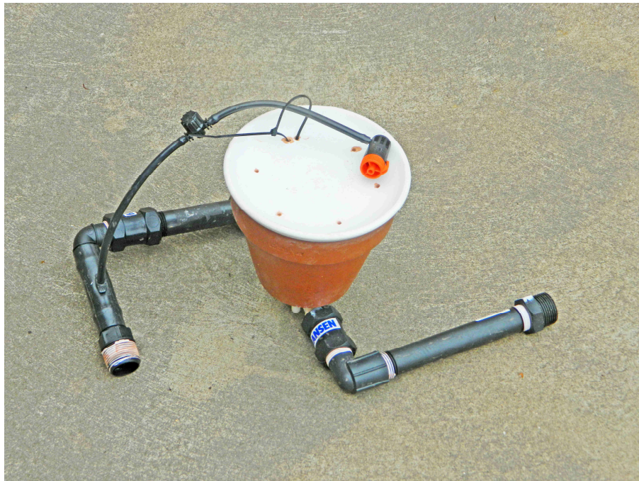
Unpowered Terracotta Irrigation Controller
