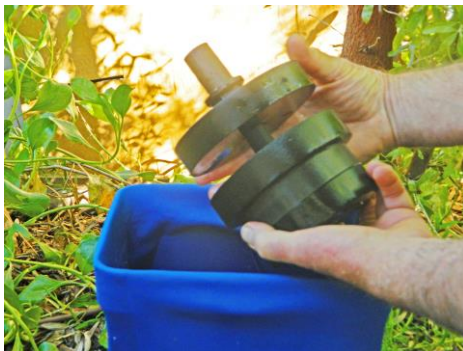
The adjustable gap between the upper and lower float determines the dripper discharge
