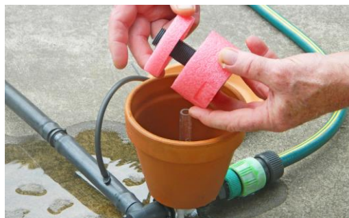
To adjust the interval between irrigation events, adjust the gap between the upper and lower float
