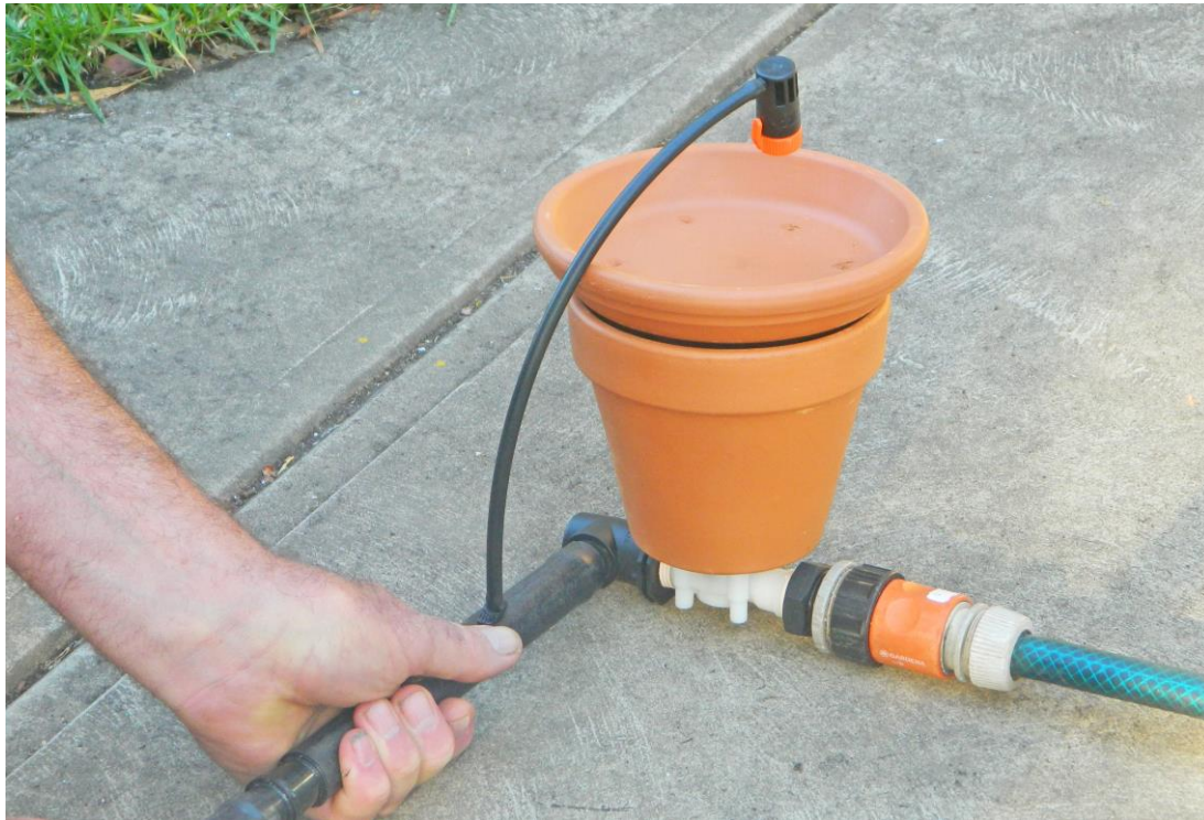
DIY Unpowered Irrigation Controller
