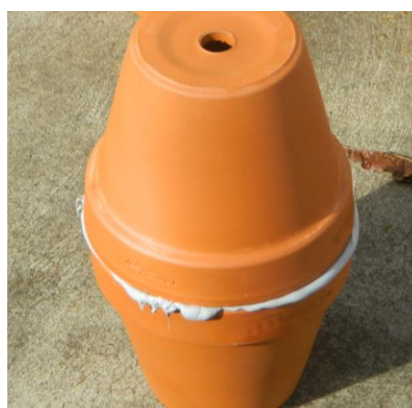
Step 4. Gently press the pots together and allow 24 hours for the sealant to cure
