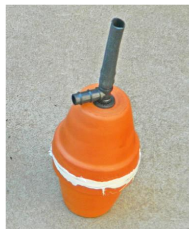
Step 4. Gently press the pots together and allow 24 hours for the sealant to cure
