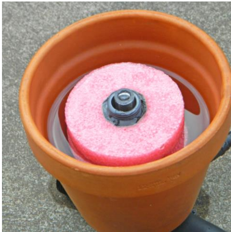
Unpowered Terracotta Irrigation Controller showing the float and the water level
