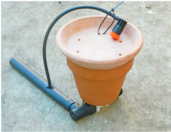
Unpowered Terracotta Valve
