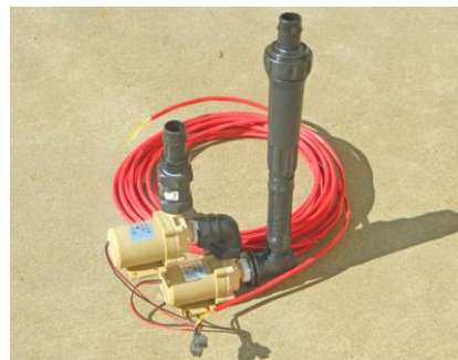
Double pump (two 19 watt pumps connected in series) with an inlet filter, fittings to connect to 19 mm poly pipe, and 9 metres of waterproof electrical cable
