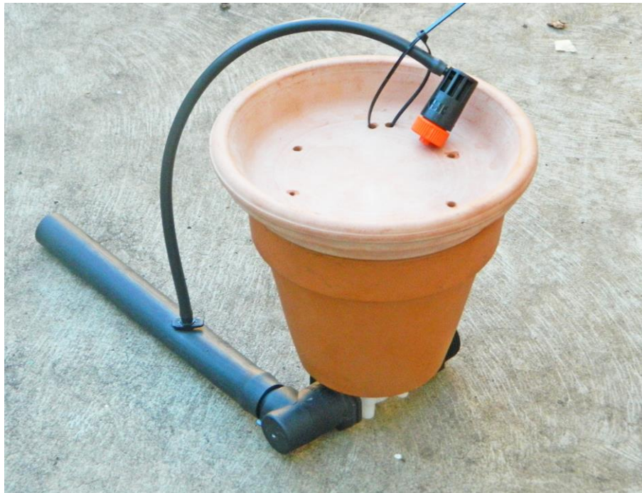
Unpowered Terracotta Valve
