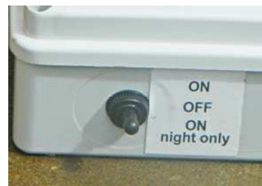
Switch in the ON night time position
