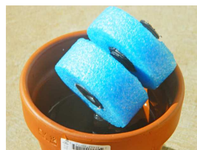
To adjust the irrigation frequency, adjust the gap between the upper and lower discs
