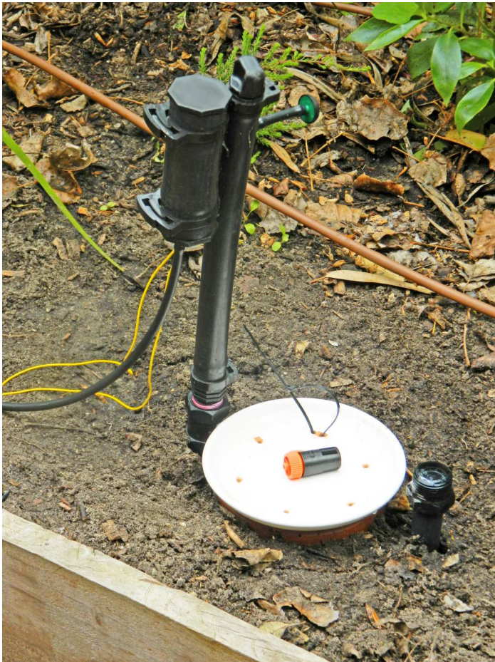
In ground installation of the Terracotta Irrigation Controller
