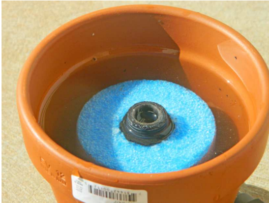
Terracotta pot showing float and water level
